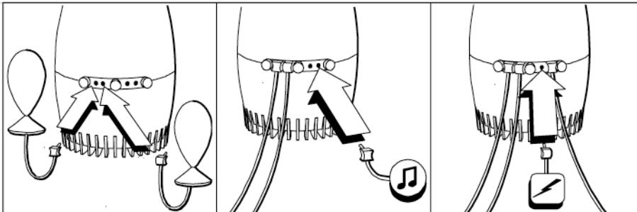
Step 2. Plug left and right satellites into position on rear of subwoofer.
